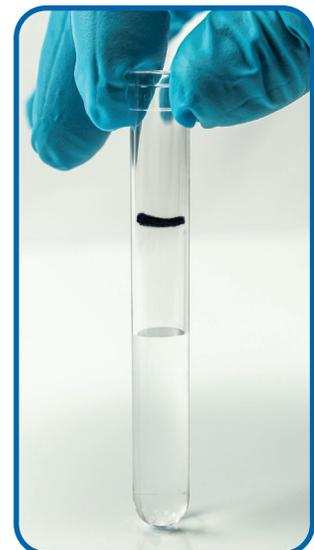
SampleSense Soil consumes < 2 mL of sample. The black line shows the original level of 5 mL extract. Post analysis 3.5 mL remains. Samples can be reanalyzed without re-extraction
